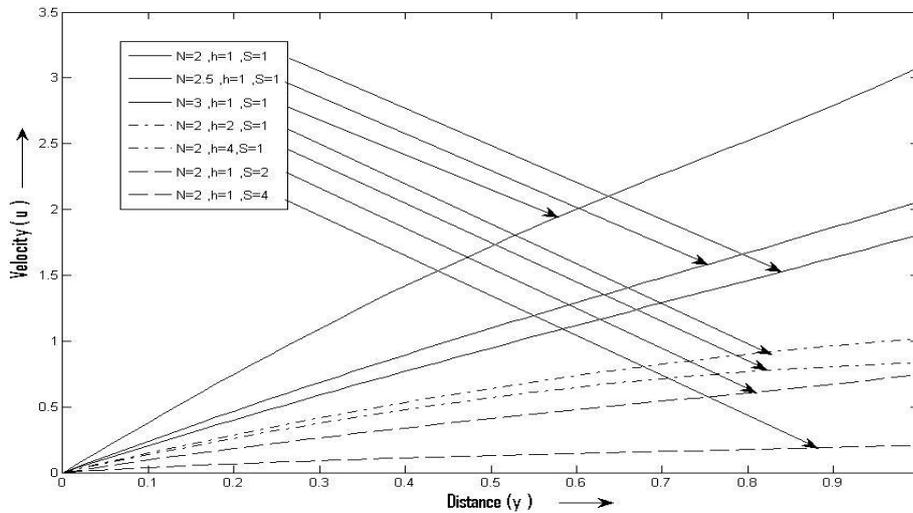
Figure 3: Effect of N, h and S on Velocity Profile when  $w=1, Re=0.71, Gr=1, t=1, Gm=1, Pe=1, H=1, \lambda=1$  and  $Sc=0.22$
