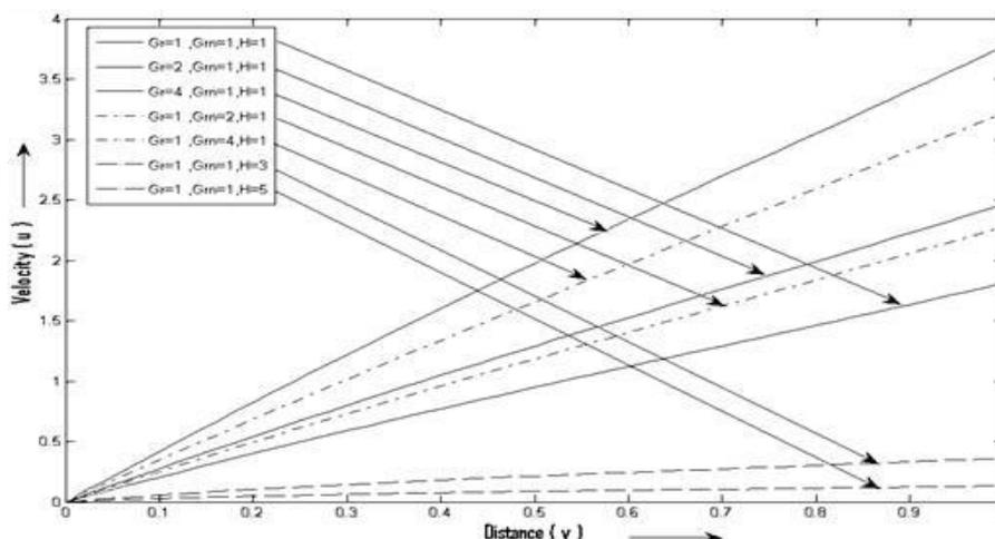
**Figure 1: Effect of  $Gr, Gm$  and  $H$  on Velocity Profile when  $\lambda=1, Sc=0.22, S=1, h=1, w=1, t=1, Re=0.71, Pe=1$  and  $N=2$**
