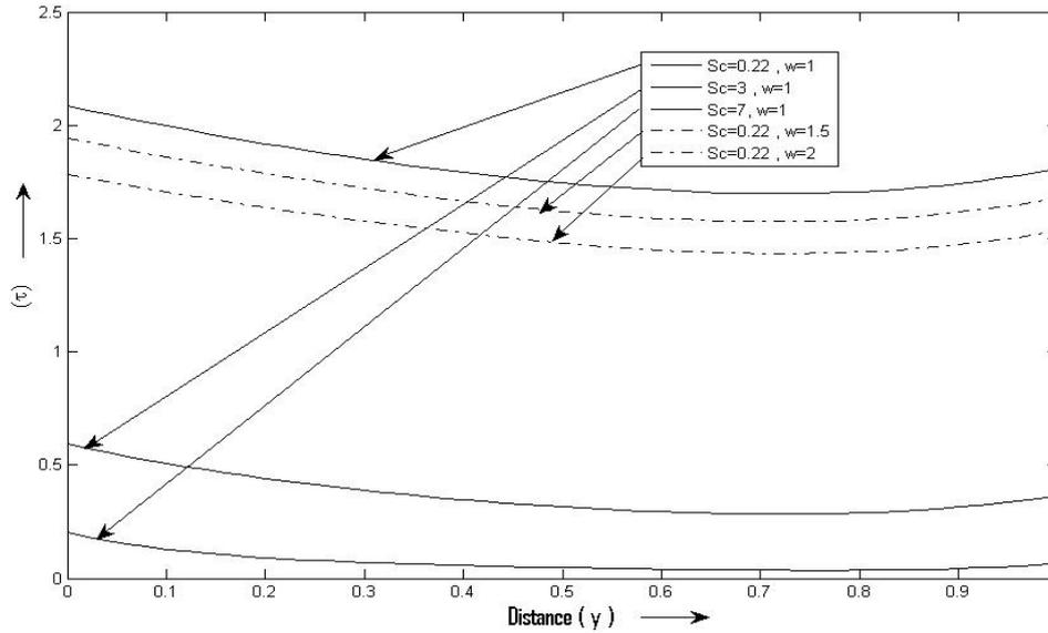
Figure 8: Effect of Sc and w on Shearing Stress when  $t=1$ ,  $Gm=1$ ,  $Gr=1$ ,  $Re=0.71$   $Sc=0.22$ ,  $Pe=1$ ,  $H=1$  and  $w=1$
