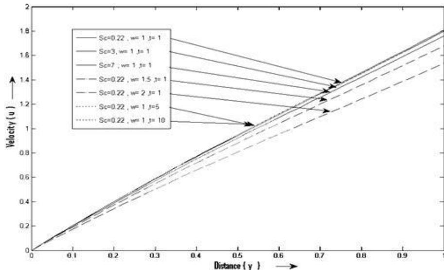
Figure 4: Effect of Sc, w and t on Velocity Profile when  $H=1, Re=0.71, S=1, h=1, w=1, \lambda=1, Gr=1, Pe=1, Gm=1$  and  $N=2$
