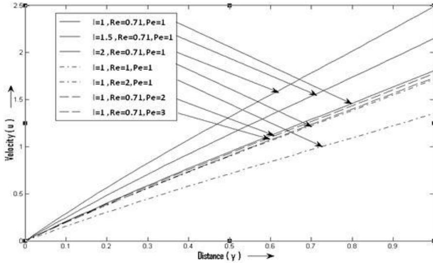
Figure 2: Effect of Re, Pe and  $\lambda^{(l)}$  on Velocity Profile when  $H=1, Sc=0.22, S=1, h=1, w=1, t=1, Gr=1, Gm=1$  and  $N=2$
