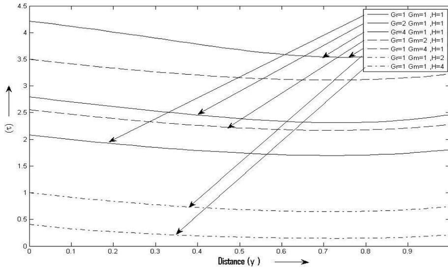
**Figure 5: Effect of Gr, Gm and H on Shearing Stress when  $t=1, Re=0.71, Pe=1, Sc=0.22, h=1, w=1, S=1, \lambda=1$  and  $N=2$**
