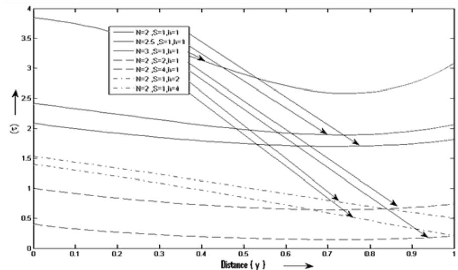
**Figure 7: Effect of N, S and h on Shearing Stress when  $t=1, Gm=1, Gr=1, Re=0.71, Sc=0.22, Pe=1, H=1$  and  $w=1$**
