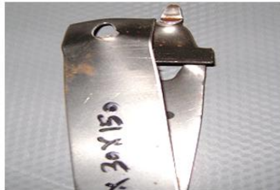
Pull Out Failure
