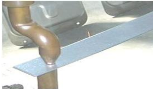
Figure 2: Specimen for Nugget Test
