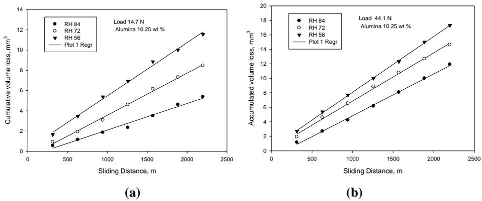
Figure 3: Cumulative Volume Loss with Sliding Distance of a Composite Material has a 31 wt% of Alumina at Different Relative Humidity at Normal Loads of (a) 14.7 N and (b) 44.1N
