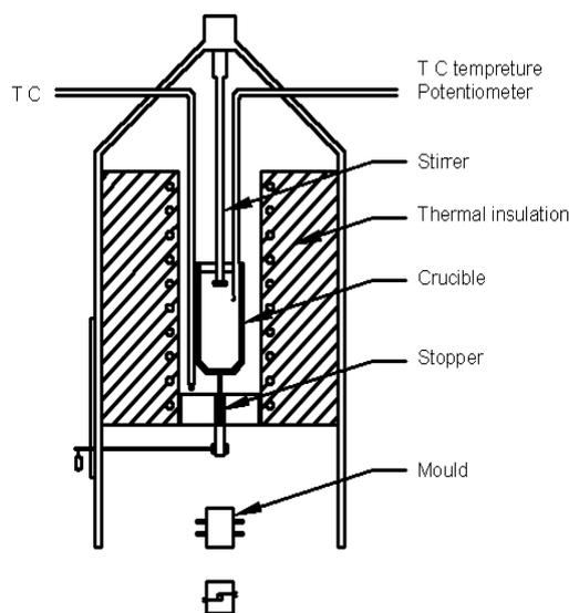
**Figure 1: Schematic Diagram Showing Experimental Set-up for Stir-Casting**
