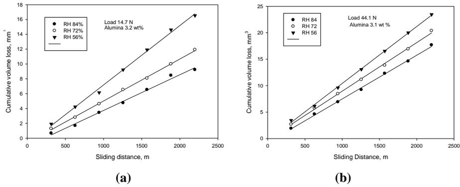
Figure 2: Effect of Relative Humidity on Cumulative Volume Loss of a Composite has 3.1 wt% of Alumina, at Normal Loads of (a) 14.7 N and (b) 44.1N
