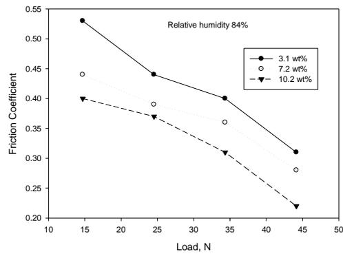
Figure 7: The Effect of Alumina Contents on the Friction Coefficients of the Composites Materials
