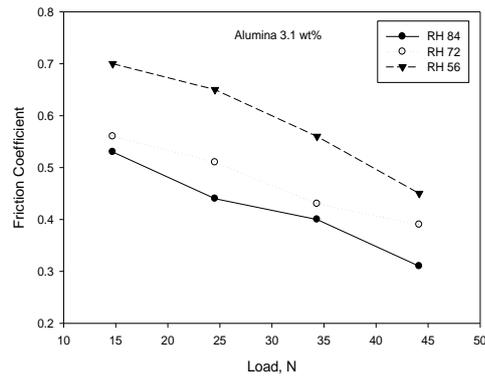
Figure 8: The Effect of Humidity on the Friction Coefficient of a Composite has 3.1wt% of Alumina
