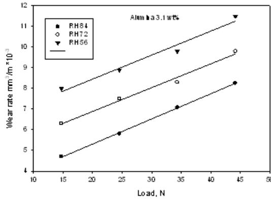
Figure 4: The Effect of Humidity on the Wear Rate of the Composite has 3.1 wt% of Alumina
