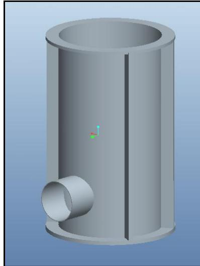
**Figure 5: Modified Design of Base Stool Cylindrical Shell**
