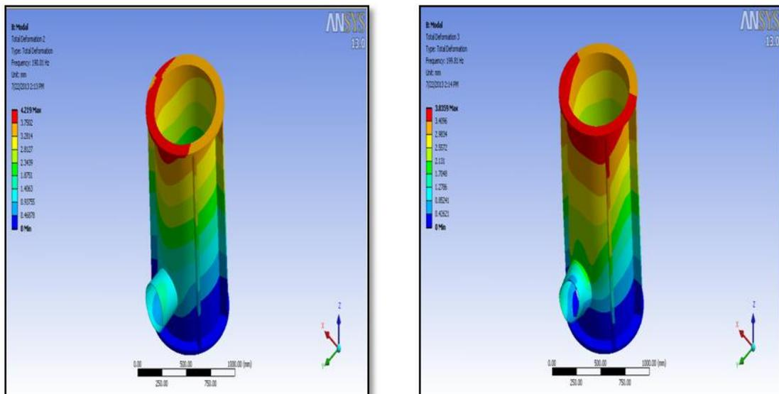
**Figure 6: First and Second Mode Shapes of Modified Design**
