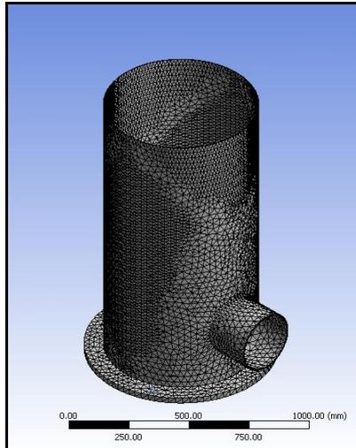
**Figure 3: Mesh Model of VTP Base Stool**
