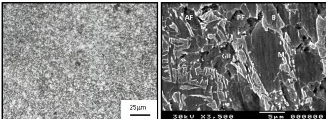
Figure 9: Water Quenched Microstructure, PF, Polygonal Ferrite; M, Martensite; AF, Acicular Ferrite; GB, Granular Bainite
