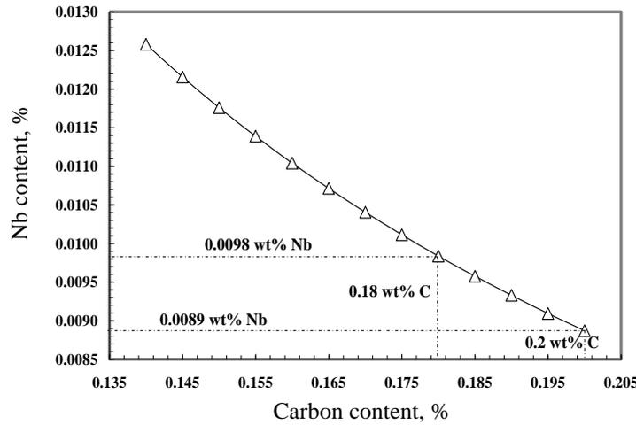
**Figure 2: Active Nb in the Presence of Different Carbon Contents with 40ppm N<sub>2</sub> and 1080°C Heating Temperature**
