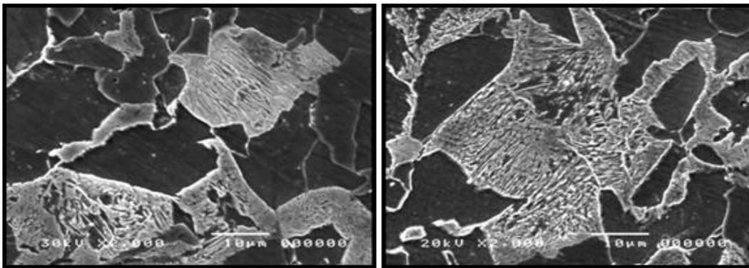
**Figure 4: Ferrite Grains with  $20\mu\text{m}$  Grain Size Surrounding Aggregates of Mixed Hard Phases**
