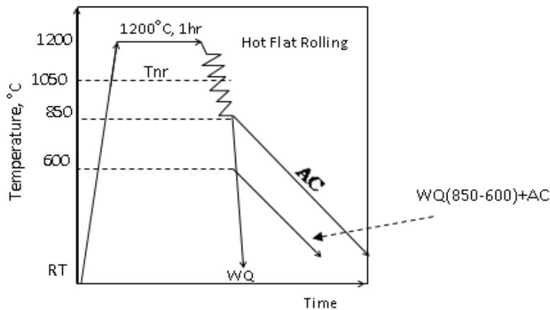
**Figure 1: Schematic Diagram of Pilot Hot Deformation Processing**
