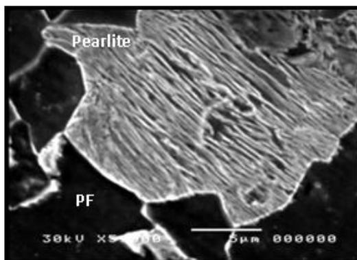
**Figure 5: Pearlite inside the Mixture of Phases Islands**
