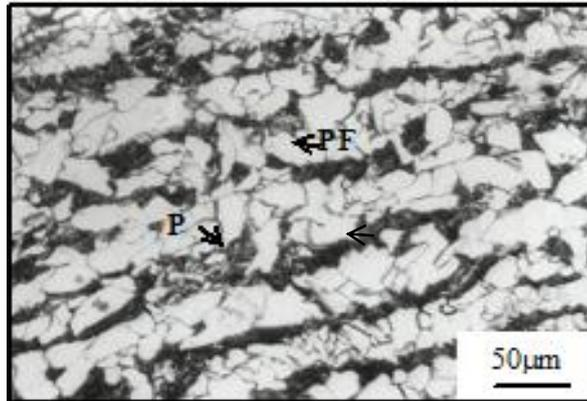
Figure 7: Ferrite – Pearlite Microstructure of Air Cooled Steel after Deformation, PF, Polygonal Ferrite; P, Pearlite
