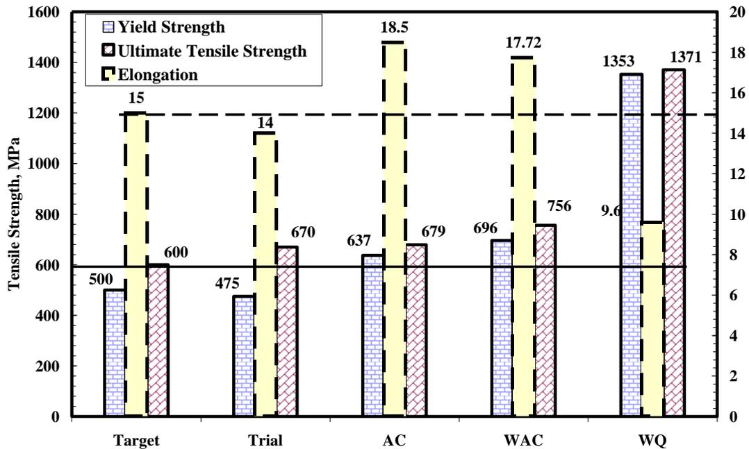
Figure 10: Tensile Properties of Steel at Different Conditions
