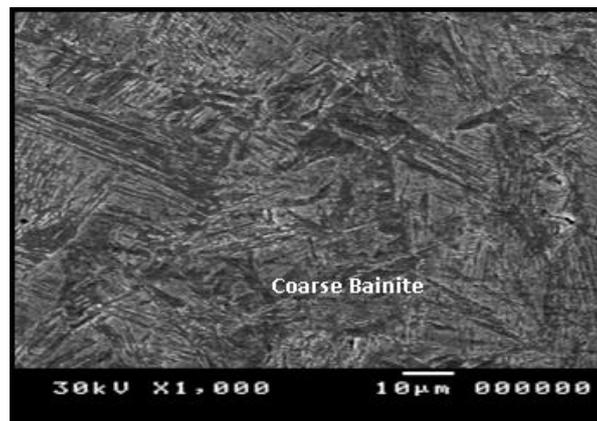
Figure 8: Water Quenching-Air Cooled Microstructure
