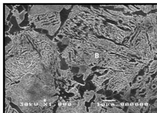
**Figure 6: Bainite inside the Mixture of Phases Islands**
