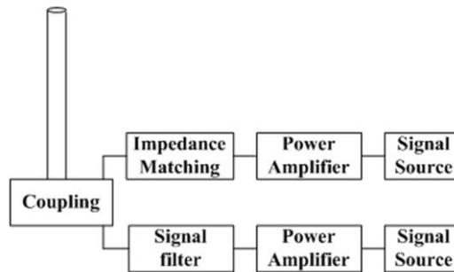
**Figure 6: The Structure of Monopole Cylindrical Plasma Antenna Excited by Surface Wave**
