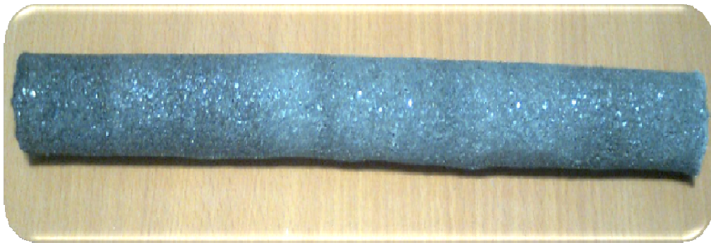
Figure 2: Sand Pack after In-Situ Gelation of PHPA-HMTA-Pyrocatechol Gel System
