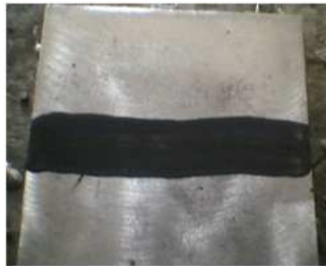
Figure 1: Schematic Representation of Activated Flux
