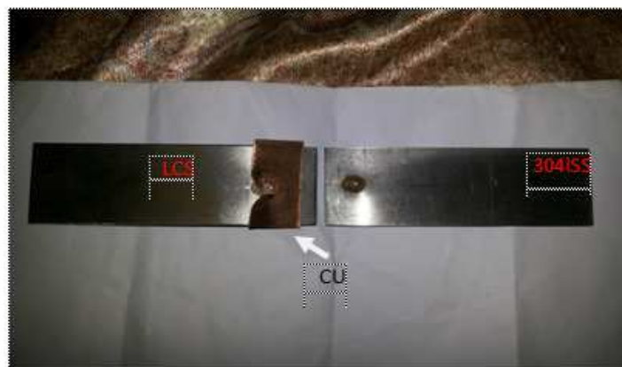
Figure 19: Interfacial Fracture Mode for Joints LCS/Cu/304LSS
