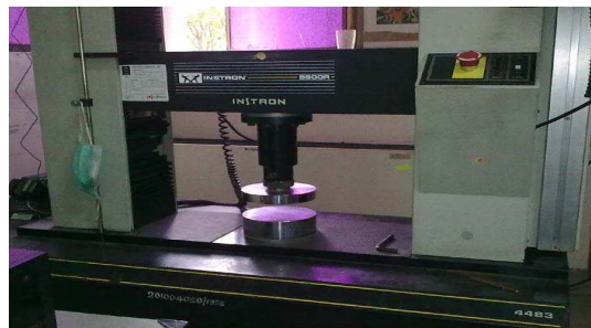
Figure 3: Universal Testing Machine (UTM) Used for Compressive Strength Testing
