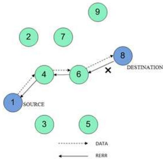
**Figure 3: Route Maintenance Stage in AODV**
