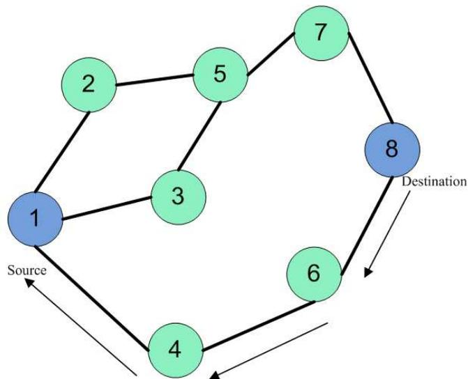
**Figure 4b: Path Taken by the Route Reply (RREP) Packet**
