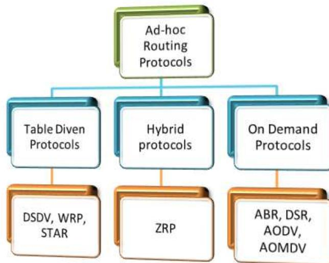
**Figure 1: Routing Protocol in MANETs- An Overview**
