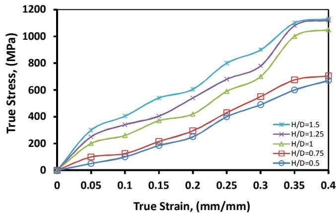
Figure 8: True Stress–Strain for Tapered Lubricated Specimens
