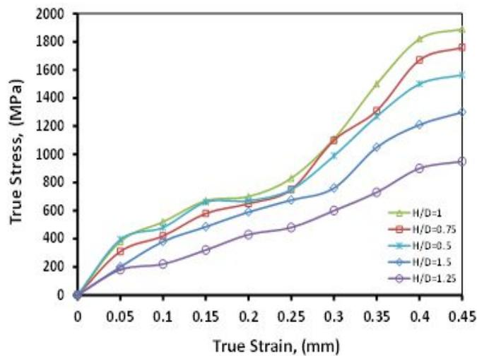
Figure 6: True Stress–Strain for Solid Lubricated Specimens
