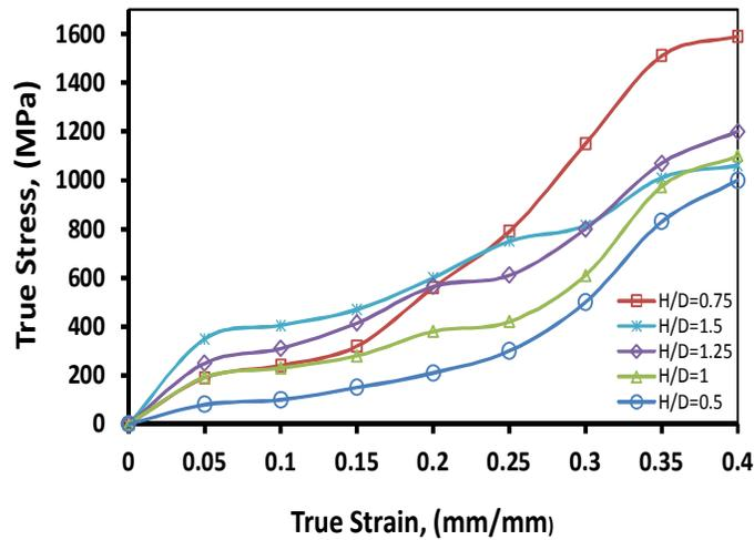
Figure 7: True Stress–Strain for Tapered Non- Lubricated Specimens
