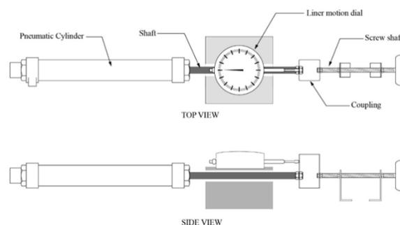
Figure 4: Top and Side Views of the Sample Cup Connected Cylinder and Fittings
