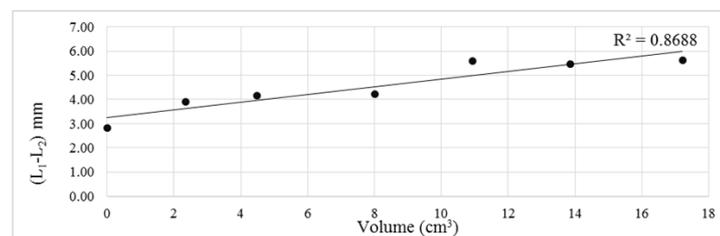
**Figure 10: Calibration Curve of the Air Pycnometer**
