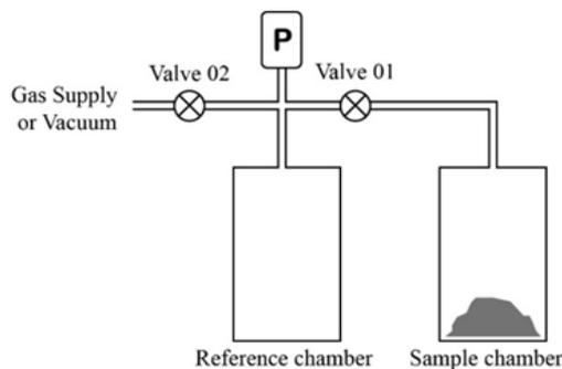
**Figure 1: Diagram of Constant Volume Pycnometer**
