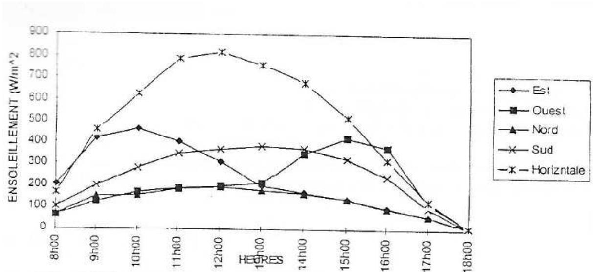
**Figure 1: Decomposition of the Solar Flux on the Faces of a Building.**
