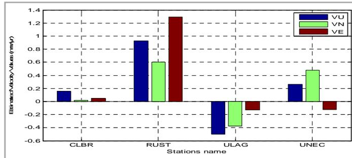
**Figure 7: The Precision Solution of Deformation and Reference Site of the Study Area in the 4th Campaign**
