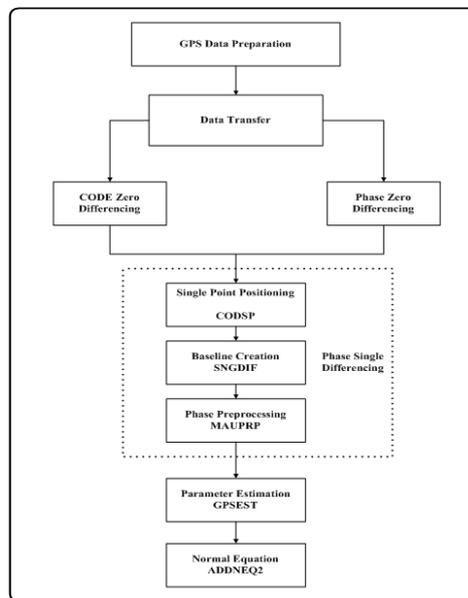
**Figure 3: Data Processing Procedure Employed in the Bernese GPS Scientific Software Version 5.0 [3]**
