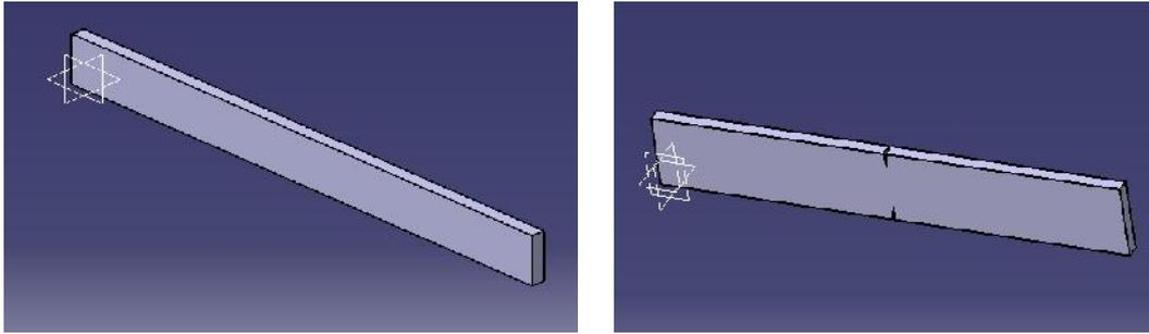
**Figure 2: CAD Model of Regular Specimen & Triangular Notched Specimen.**
