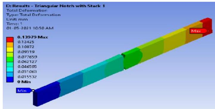
**Figure 6: Deformation Result of Triangular Notched Specimen.**
