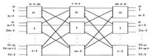
Fig. 1: A Basic General Clos Interconnection Network
