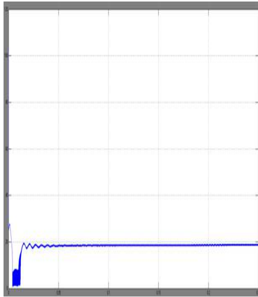
Figure 16 Pv Mppt Charger Input Voltage
