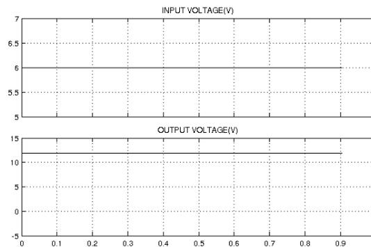
**Fig 10. Output Voltage Maintained Constant When the Input Given is 6V Converter Acts in Boost Mode**
