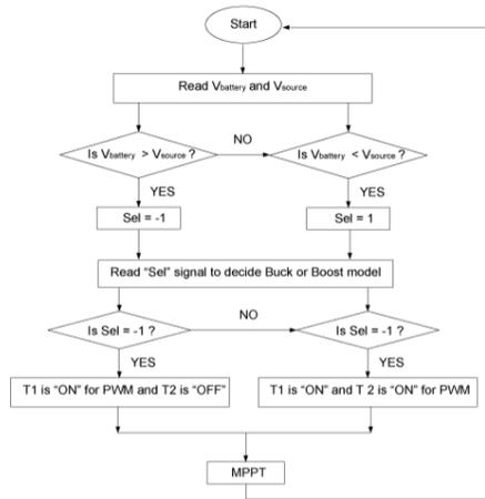
**Fig 5. Flow Chart of Buck/Boost -Mode Selector**
