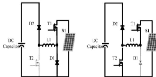
**Fig 2.A) Buck Operation (B) Boost Operation**
