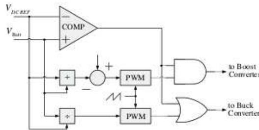
**Fig 6. Control Circuit for Wind Generation and Fuel Cell**
