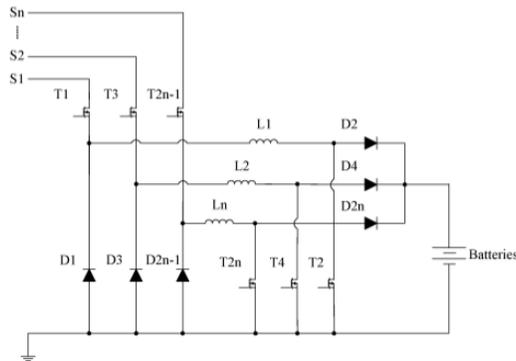
**Fig 3. Multiple Input Topology**
