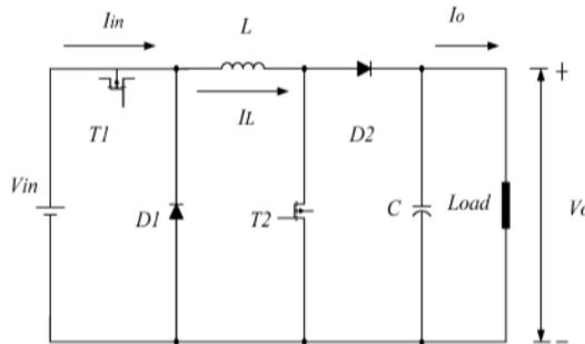
**Fig.1 The Configuration of Non-Inverting Dc/Dc Converter**
