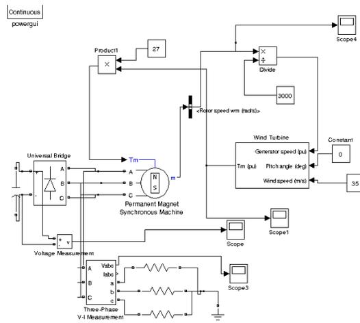
Fig 11. Wind Energy System with PMSM
