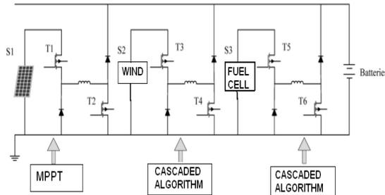
**Fig. 7 Block Diagram of Proposed System**
