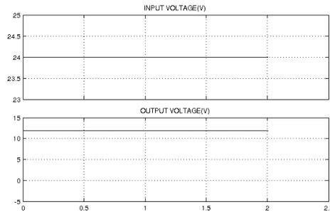
**Fig 11. Output Voltage Maintained Constant When the Input Give is 24V-Converter Acts as Buck Converter.**
