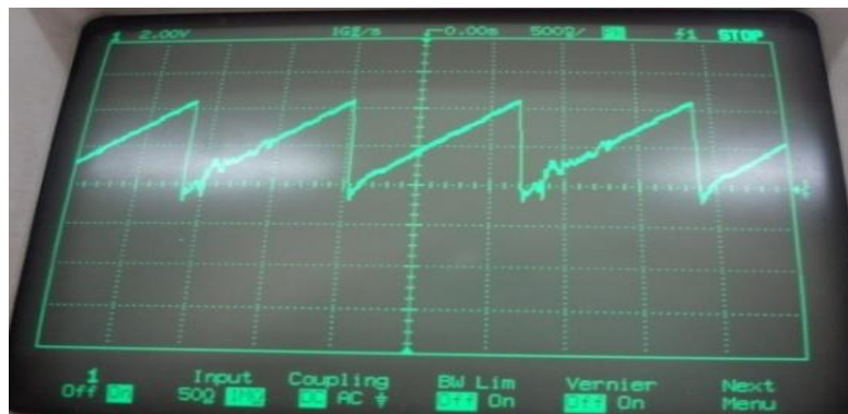
Figure 15: Ramp Voltage Across COSC Under Load Condition
