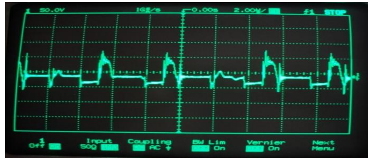
Figure 17: Drain Waveform under Load Condition
