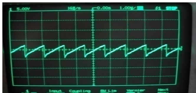
Figure 12: Ramp Voltage Across C_{OSC} at No Load
