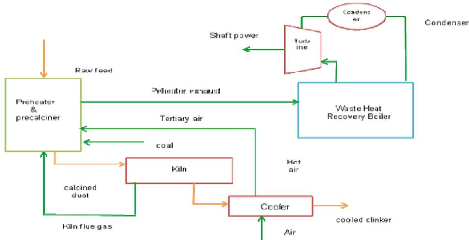
**Figure 3: Waste Heat Recovery System**
