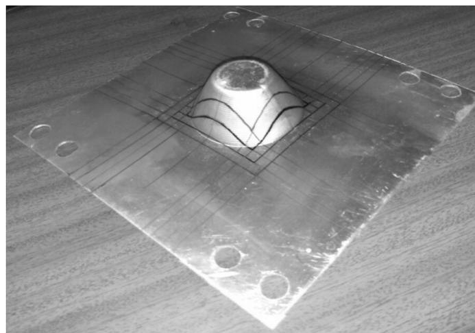
**Figure 5: Conical Cup drawn on CNC Machine**
