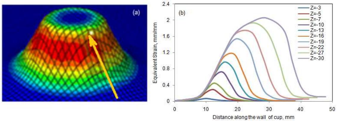
Figure 6: Major Strain Induced during SPIF Process: (a) FEM Result and (b) Experimental Result
