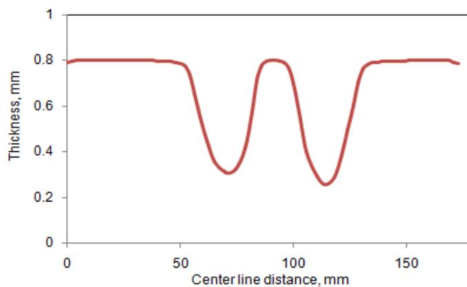
Figure 8: Thickness Variation along the Walls of Conical and Pyramidal Cups
