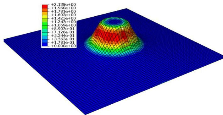
**Figure 4: Major Strain Induced in Conical Cup**
