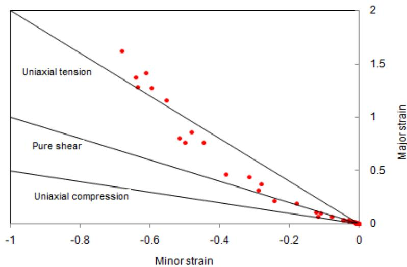
Figure 7: Formability Limit Diagrams of Conical and Pyramidal Cups
