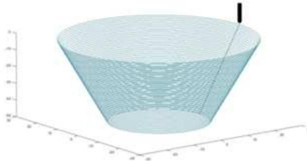
**Figure 2: Tool Path Generation**
