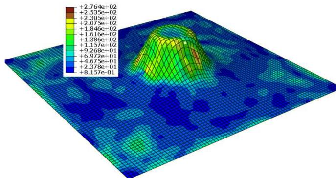
**Figure 3: Equivalent Stress Induced in Conical Cup**
