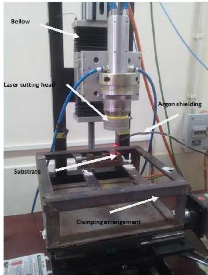
**Figure 4: Experimental Setup for Laser Cladding**
