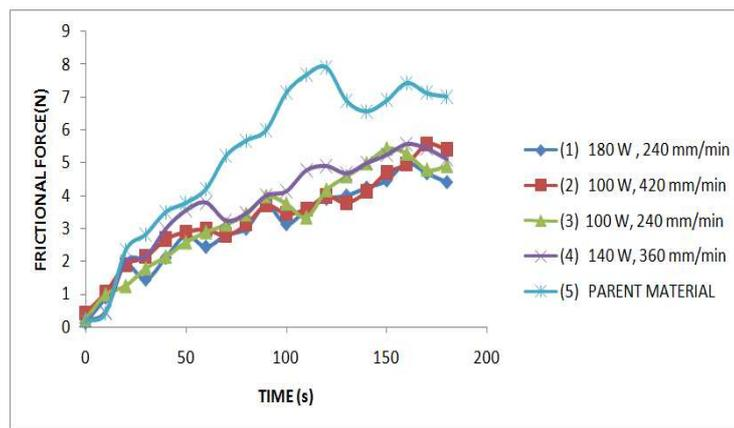
**Figure 12: Variation in the Frictional Force of Laser Cladded Ni-WS<sub>2</sub>-Al<sub>2</sub>O<sub>3</sub> Surface with Time**
