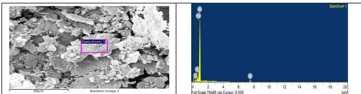
**Figure 1: Morphology and Chemical Composition of Ni Powder**
