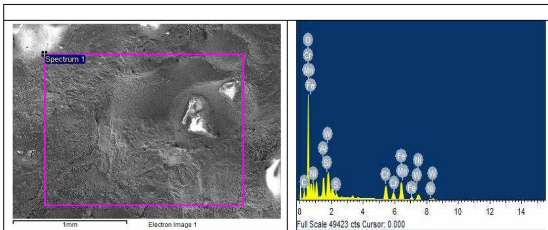
Figure 9: EDAX Image of Worn Surface Cladded at 180W and 240mm/min
