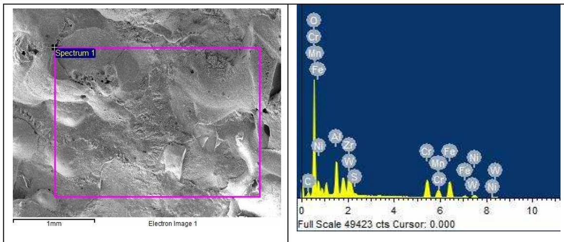
Figure 10: EDAX Image of Unworn Sample Cladded at 140W and 360 mm/min
