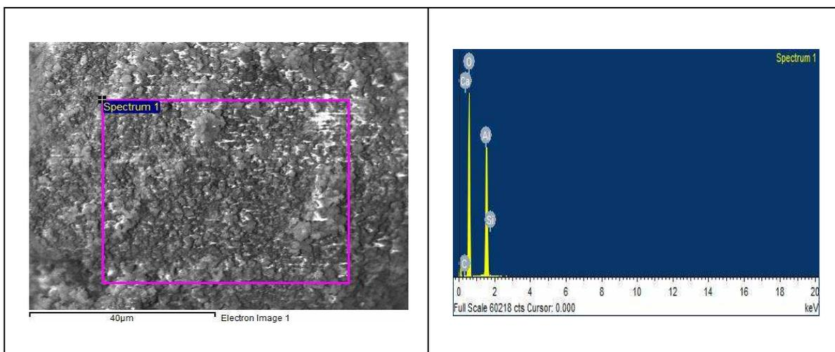
Figure 3: Morphology and Chemical Composition of  $Al_2O_3$  Powder
