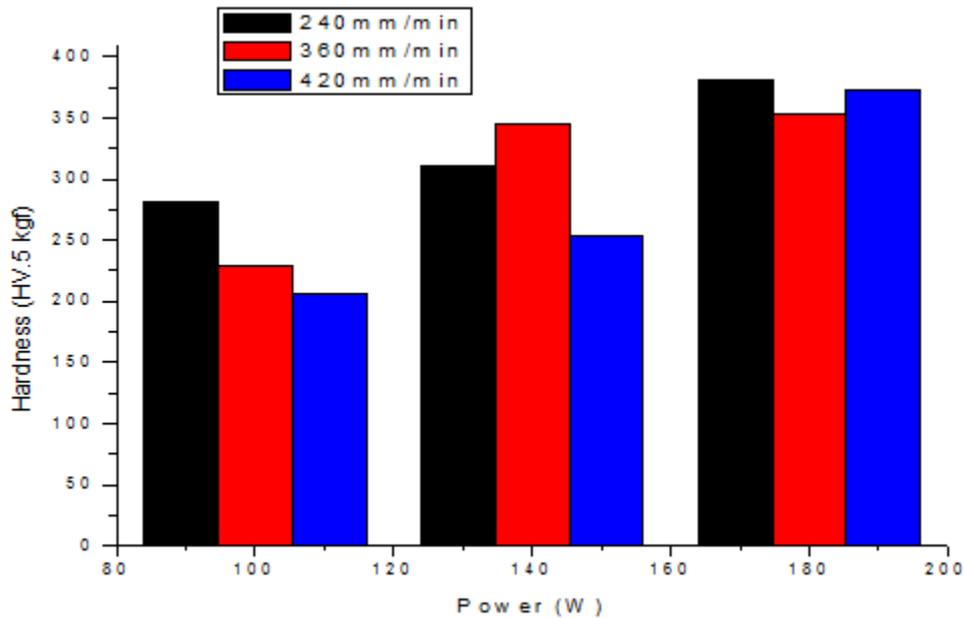
**Figure 13: Microhardness Profile of Laser Clad Ni-WS<sub>2</sub>-Al<sub>2</sub>O<sub>3</sub> Coatings**
