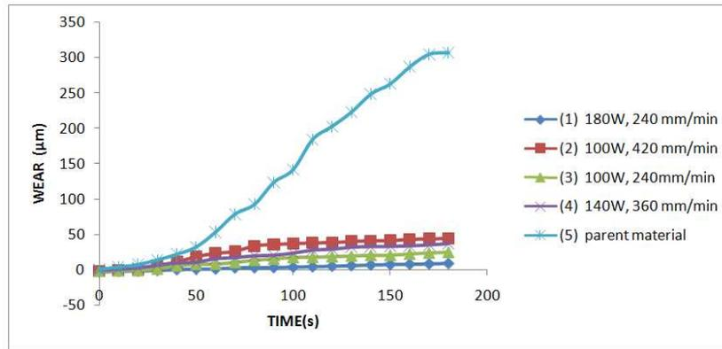
**Figure 11: Variation in the Wear Rate of Laser Cladded Ni-WS<sub>2</sub>Al<sub>2</sub>O<sub>3</sub> Surface with Time**
