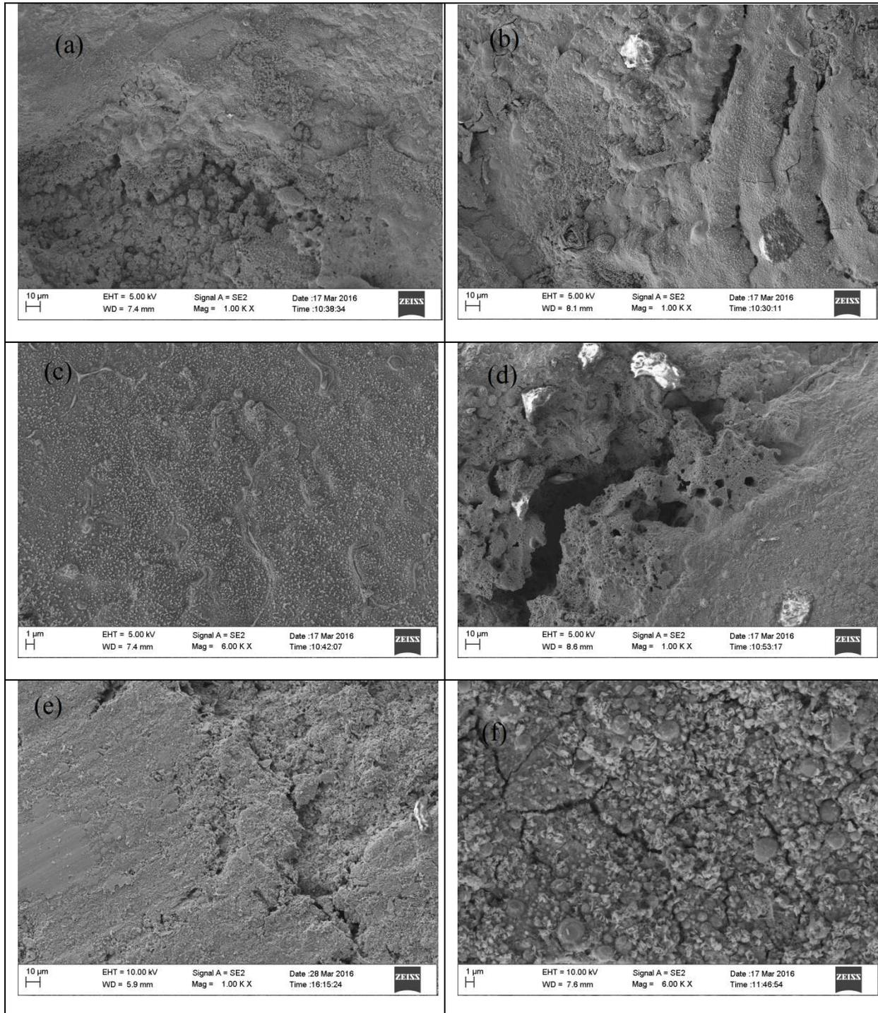
**Figure 8: FESEM Micrographs of Untested and Tested Surfaces: (a) and (b) at 180W and 240 mm/min,(c) and (d) at 140W and 360mm/min,(e) and (f) at 100W and 240 mm/min**
