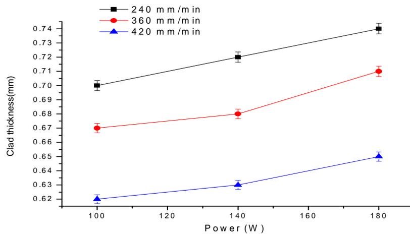
Figure 7: Variation of Clad Thickness with Power and Speed
