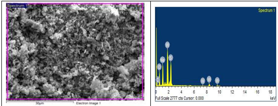
Figure 2: Morphology and Chemical Composition of  $WS_2$  Powder
