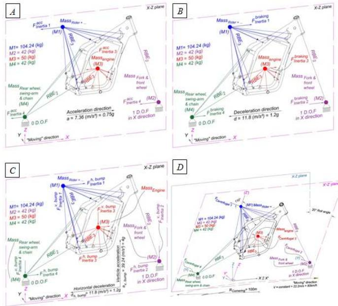
A: acceleration, B: braking, C: bumping, & D: cornering
