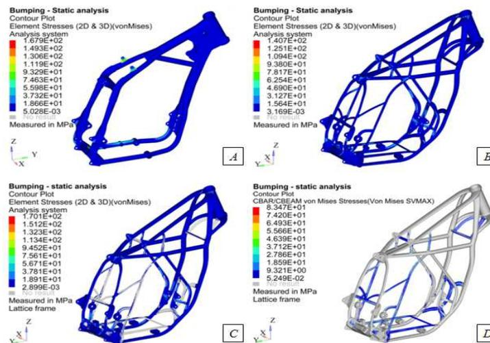
**Figure 4: Equivalent Stress Distribution Predicted in: A: original design, B: redesigned tubular frame, C and D: redesigned tubular frame with lattice**
