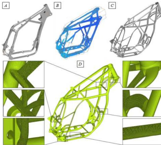
**A: Original Frame, B: New Concept, C: Redesigned Frame, D: Tubular Lattice Frame**
