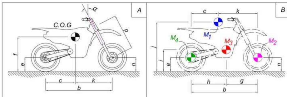
**A: Motorcycle with its Centre of Gravity (C.O.G), B: Substituted Masses of Motorcycle**
