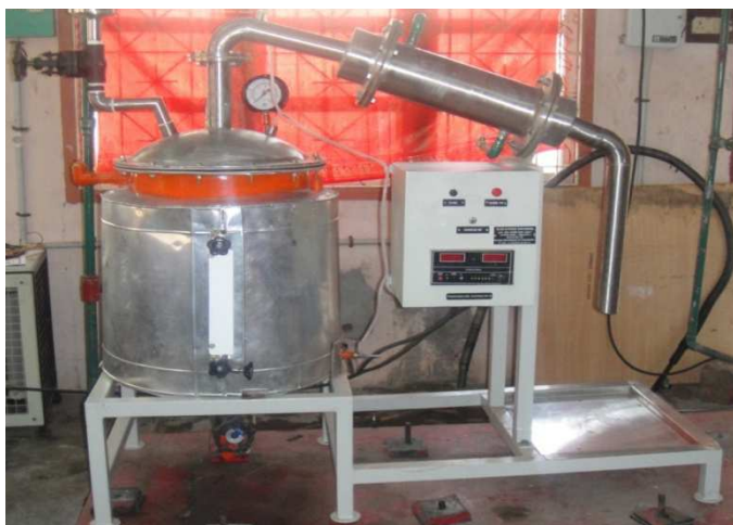
Figure 5: Low Boiling Hydrocarbons Separating System
