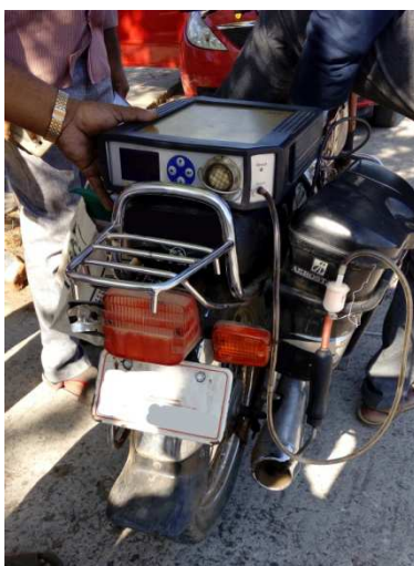
Figure 6: AVL Di-Gas Analyser Fitted in Test Engine Exhaust Silencer
