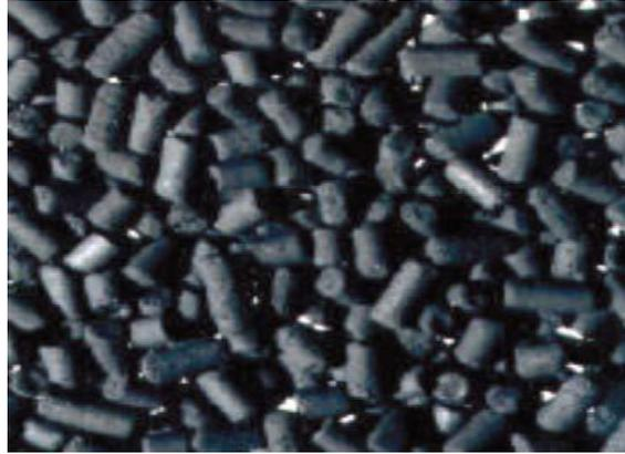
**Figure 2: Carbon Molecular Sieve**
