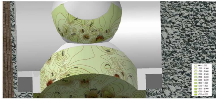
Figure 7: The Convex Part upon the Back Surface, (the Maps were Made with ARC GIS 2010 and the Depiction of the Maps was Made upon the Model, by the Use of the AUTOCAD 2012) the Legend is the same for all the Maps Showing, the Ultrasound Velocities V_p (m/sec)
