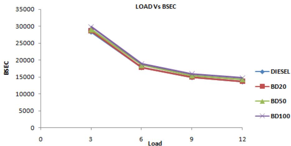
**Figure 4: The Variation of Brake Specific Energy Consumption (BSEC) with Different Engine Load for Ethanol-Biodiesel Blends and Pure Diesel Fuel**
