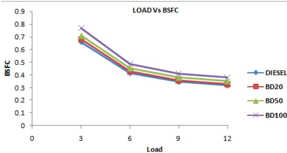
**Figure 3: The Variation of Brake Specific Fuel Consumption (BSFC) with Different Engine Load for Ethanol-Biodiesel Blends and Pure Diesel Fuel**
