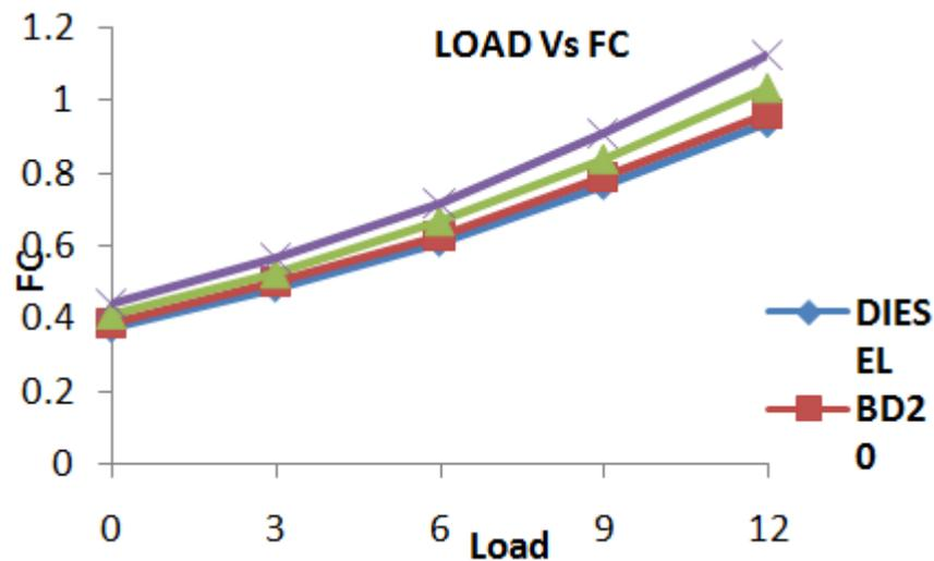
**Figure 2: The Variation of Fuel Consumption (FC) With Different Engine Load for Ethanol-Biodiesel Blends and Pure Diesel Fuel**
