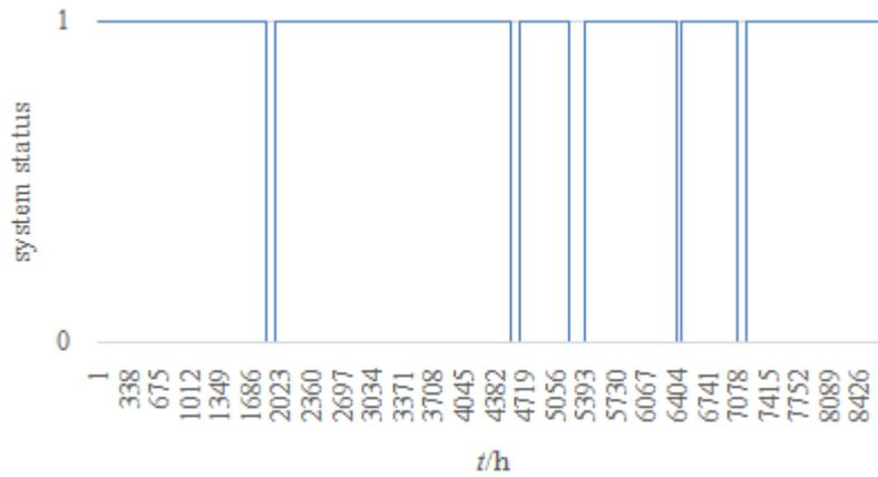
**Figure 4: Photovoltaic Generating Unit Operating Status Curve.**
