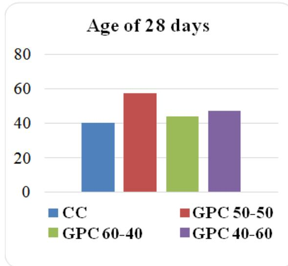
Figure 1: Compressive Strength Comparative Chart
