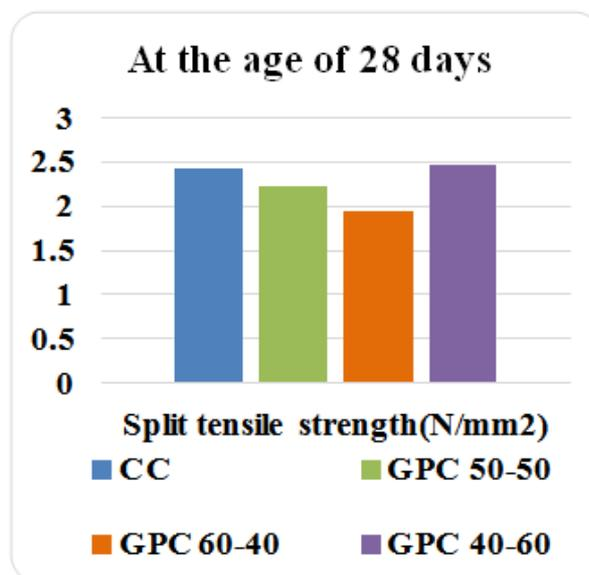
Figure 2: Split Tensile Strength Comparative Chart
