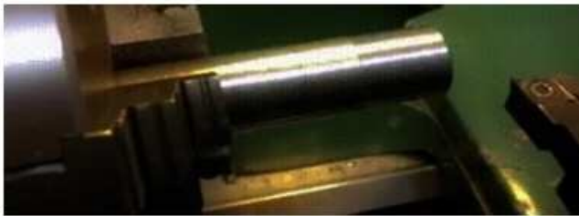
a. Creating a Surface Utilizing a Turning Tool
