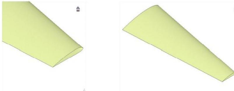
**Figure 6: No Winglets or Wingtip Devices at End Section.**
