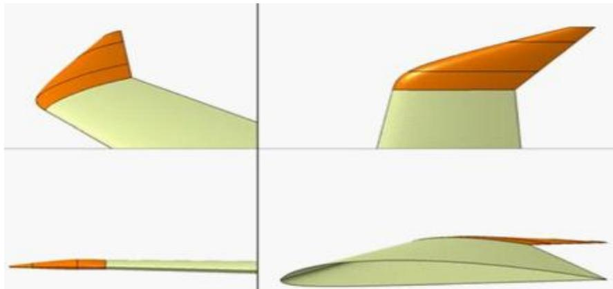
**Figure 8: Raked Wing Tip with Three Panels.**
