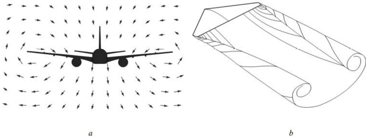
**Figure 11: (a) flow Pattern of the Velocity (b) Vortex Sheet from Trailing Edge.**
