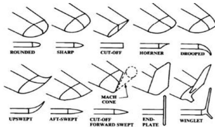
Figure 4: Different Types of Tip Devices.
