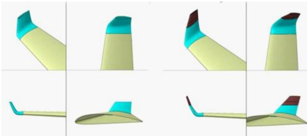
**Figure 7: Blended Winglet: (a) Blended Base; the Base Panels Placed Upon Base.**
