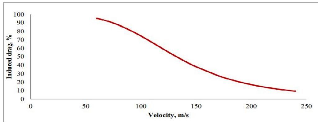
**Figure 5: Induced Drag Percentage of the Aircraft Wing Against the Velocity, m/s.**
