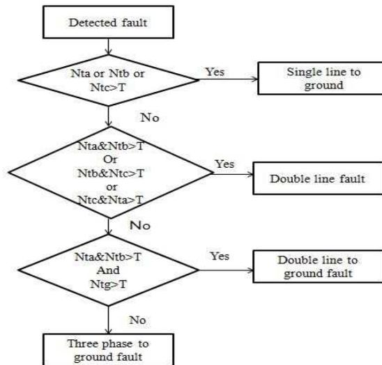
**Figure 4: Flow Chart for Fault Classification.**
