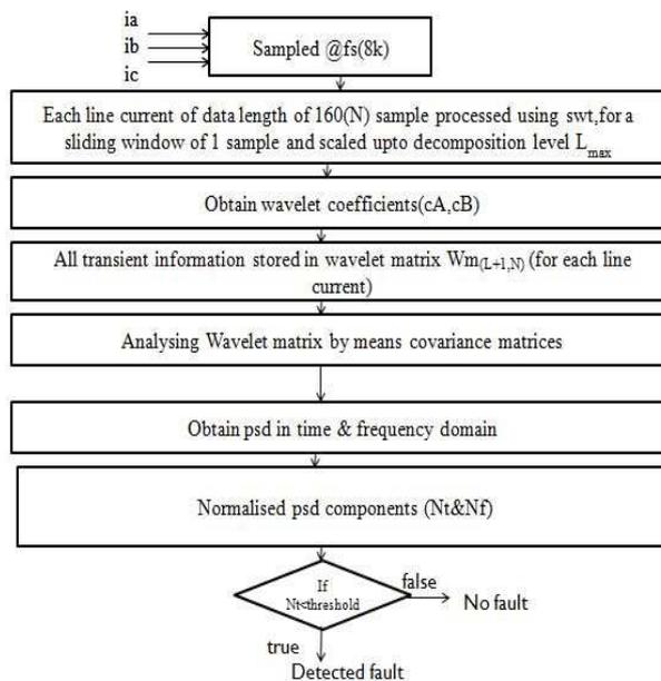
**Figure 3: Flow Chart for Fault Detection.**
