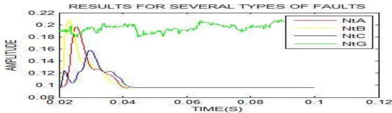
**Figure: 6(d): 3F Fault with  $R_f=50$ .**
