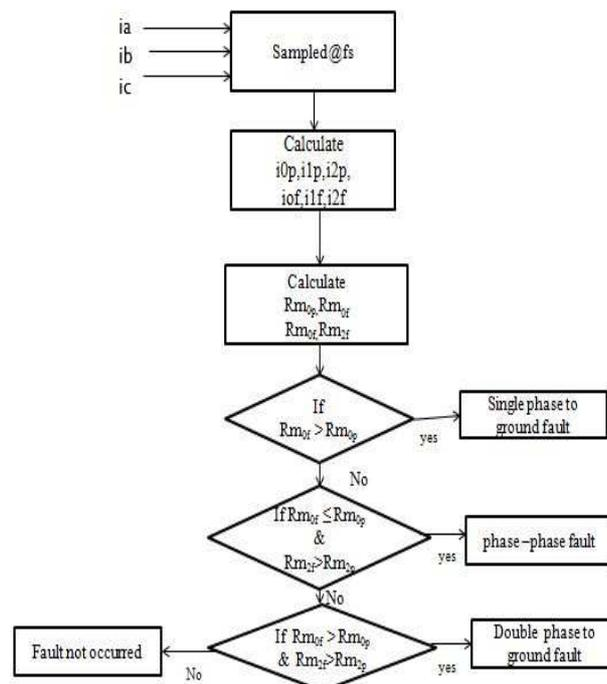
**Figure 1: Block Diagram of Classification Algorithm.**
