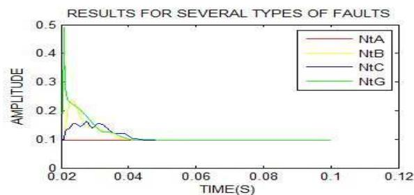
**Figure 6(c): 2F-g Fault with  $R_f = 20$ .**
