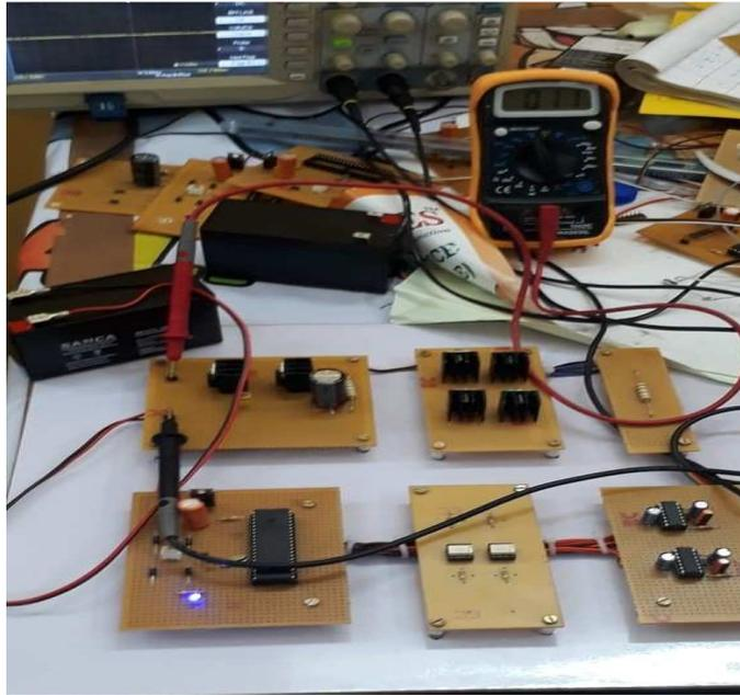
**Figure 5: Prototype of the Proposed Novel Multilevel Bi-Directional Grid Connected Inverter.**
