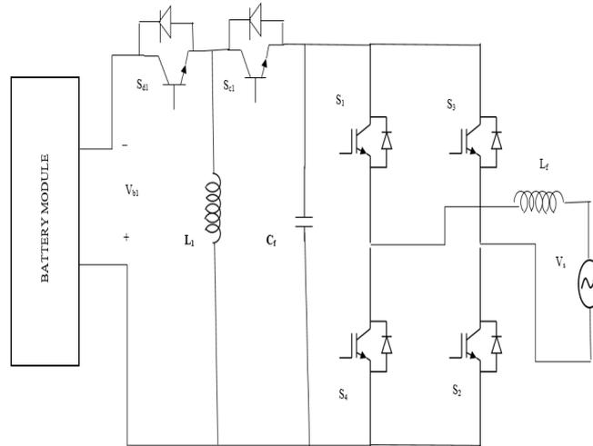
**Figure 2: Circuit Diagram of the Proposed Novel Multi Level Bidirectional Grid-Connected Inverter.**
