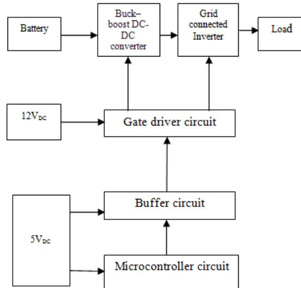
**Figure 1: Block Diagram of the Proposed System for Single Battery Modul.**
