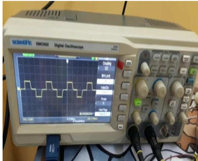
**Figure 4. Output Voltage Waveform during Battery Discharging Operation.**
